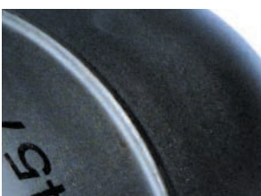
A perfectly homogeneous welding seam.
